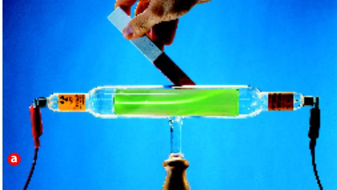
**Figure 4.5** Thomson examined two ways that a cathode ray can be deflected: **a** by using a magnet, and **b** by using electrically charged plates.
