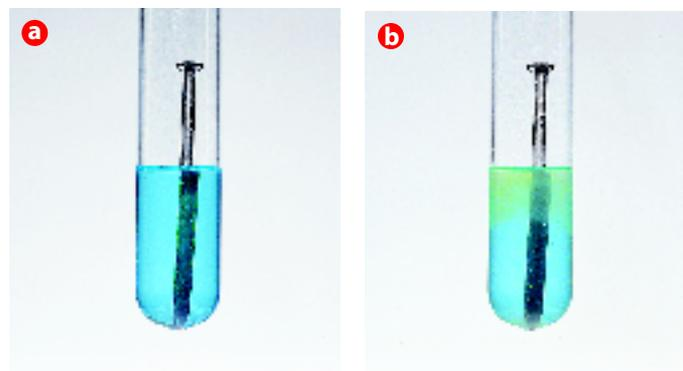
**Figure 20.14** A redox reaction occurs between iron and copper. **a** An iron nail dipped in a copper(II) sulfate solution becomes coated with metallic copper. **b** The iron reduces  $Cu^{2+}$  ions in solution and is simultaneously oxidized to  $Fe^{2+}$ .
