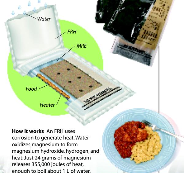
**How it works** An FRH uses corrosion to generate heat. Water oxidizes magnesium to form magnesium hydroxide, hydrogen, and heat. Just 24 grams of magnesium releases 355,000 joules of heat, enough to boil about 1 L of water.
