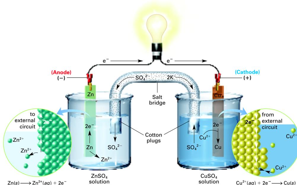
**Figure 21.3** In this voltaic cell, the electrons generated from the oxidation of Zn to  $\text{Zn}^{2+}$  flow through the external circuit (the wire) into the copper strip. These electrons reduce the surrounding  $\text{Cu}^{2+}$  to Cu. To maintain neutrality in the electrolytes, anions flow through the salt bridge.
