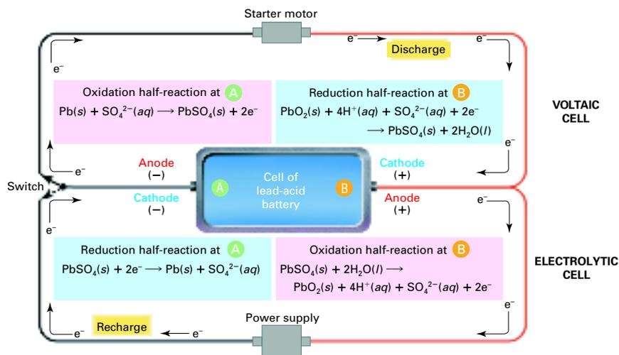
**Figure 21.6** The lead-acid battery in an automobile acts as a voltaic cell (top) when it supplies current to start the engine. Some of the power from the running engine is used to recharge the battery which then acts as an electrolytic cell (bottom). You will learn more about electrolytic cells in Section 21.3.
