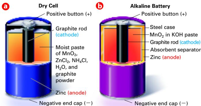
**Figure 21.4** Both dry cells and alkaline batteries are single electrochemical cells that produce about 1.5 V. **a** The dry cell is inexpensive, has a short shelf life, and suffers from voltage drop when in use. **b** The alkaline battery costs more than the dry cell, has a longer shelf life, and does not suffer from voltage drop. **Inferring** What is oxidized in these cells and what is reduced?
