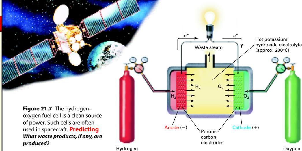
**Figure 21.7** The hydrogen–oxygen fuel cell is a clean source of power. Such cells are often used in spacecraft. **Predicting** What waste products, if any, are produced?
